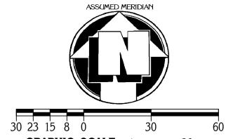
**GRAPHIC SCALE:** 1<sup>(\*)</sup> EQUALS 30<sup>(\*)</sup> O-DENOTES 5/8" (DIAMETER) x 30" (LONG) IRON PIN WITH YELLOW PLASTIC CAP BEARING "KOSIE P.S. 8167" SET
