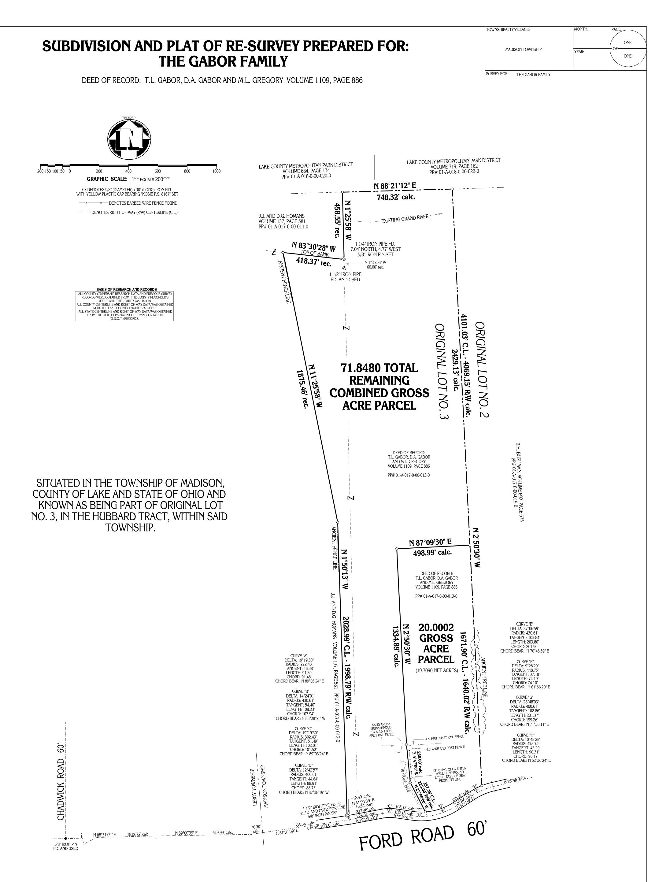
MONUMENTS WERE FOUND OR SET AS INDICATED HEREON. DISTANCES ARE IN U.S. FEET WITH DECIMAL PARTS. BEARINGS ARE TO TRUE NORTH USING NAD83 AUGUST 2004.
