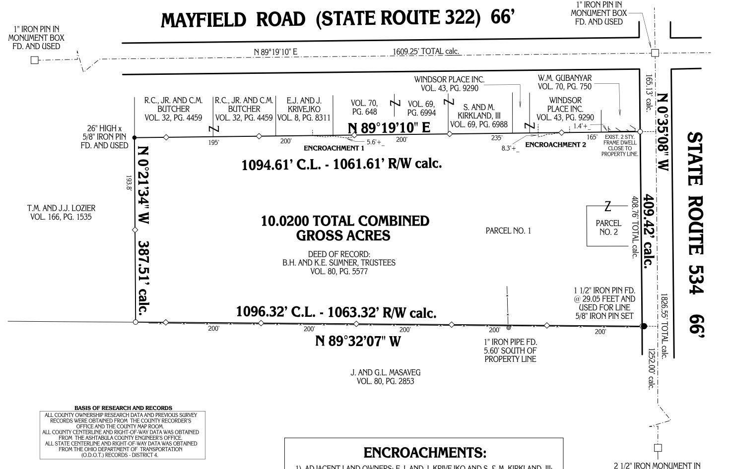
MONUMENTS WERE FOUND OR SET AS INDICATED HEREON. DISTANCES ARE IN U.S. FEET WITH DECIMAL PARTS. BEARINGS ARE TO AN ASSUMED MERIDIAN AND INDICATE ANGLES ONLY.
